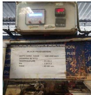
Online Ph meter & Timer for Trivalent Black Passivation
