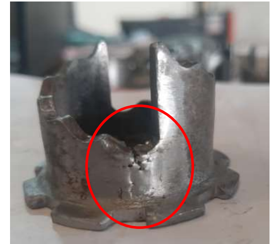
Welding pin hole
