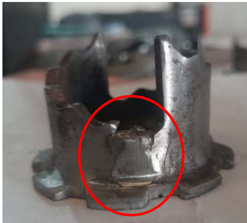
Excess welding ,buffing step
