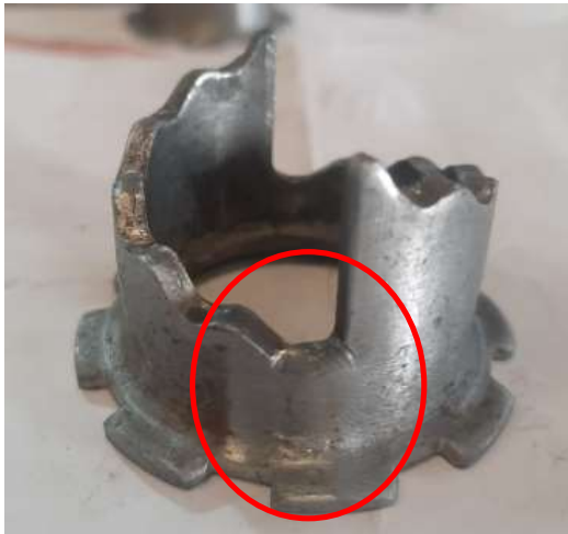
Excess welding ,buffing step
