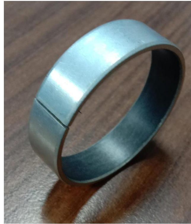
Part Tin Plated (Flash completed)
