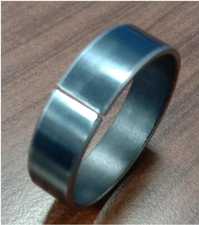
Part before Tin plating (Tin Flash)
