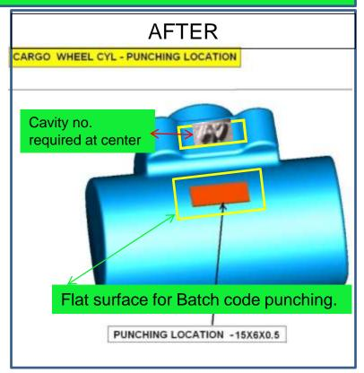
To resolve batch code punching depth uniformity issue Punching pad (15\*6\*0.5) will be provided and Cavity No. at center as per above Image.
