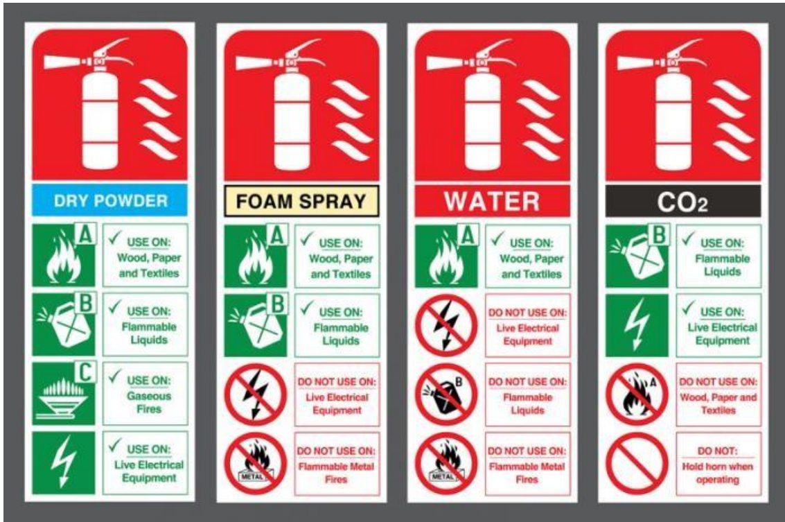
Figure 3 : Use of Right Fire Extinguisher
