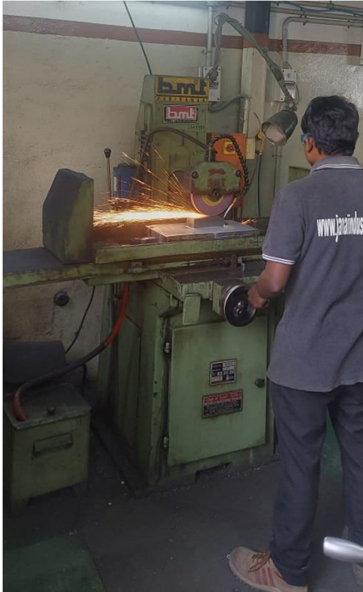
Surface Grinding Machine No 13
