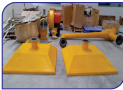
FRP Fume Extractors
