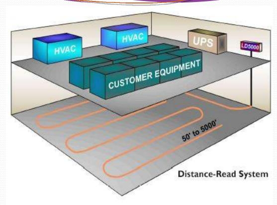
Any leakage in the premises due to air condensation or due to any other reasons will be detected by water leakage detection cables laid out to cover the corners and other vulnerable areas this can be installed in Data Centers.
