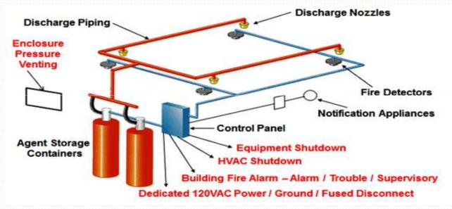
Novec Systems are used in Data Center areas and electrical areas to suppress fire using Clean Agents. Less environmental friendly systems called as FM200 are used in Premises where there is a possibility of Human presence more often than not. Gas calculations are as per Premise Dimensions.
