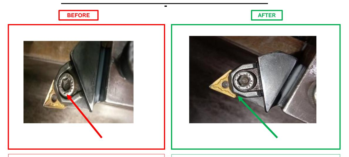
Insert clamping nut head got damaged hence unable to do the proper tightening where earlier replacement Frequency was 5000 Nos./Nut Nut changed frequency reduced by 20 % From 5000 Nos./nut to 4000 Nos./Nut
