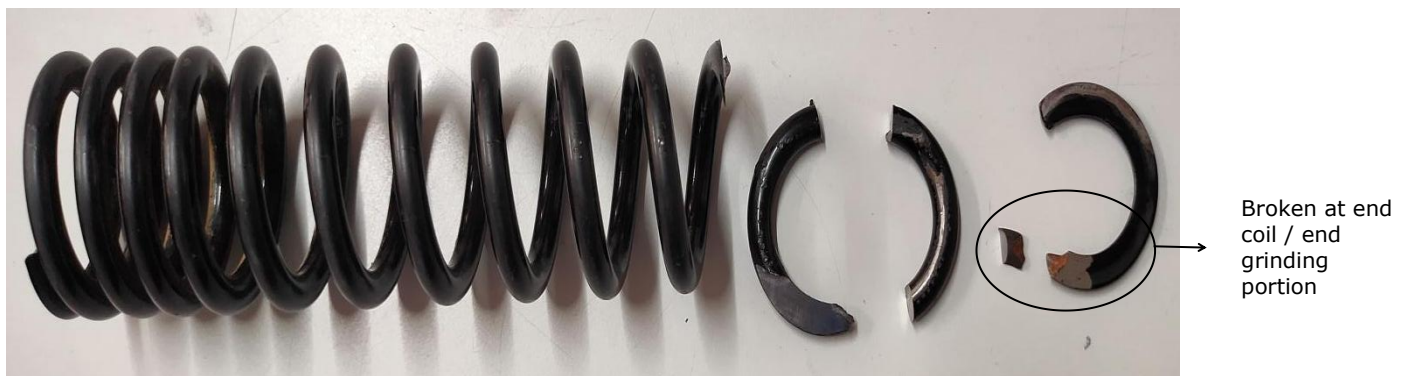
Photograph 1: As received photograph of the broken spring and broken at end coil from one end.
