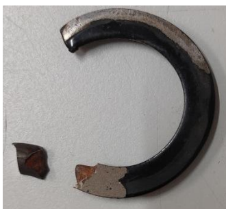
Photograph 11,12 and13: Fracture face found to rusty in condition and adjacent coil found to be with extensive mechanical damage/worn out and powder coating peeled off in condition.
