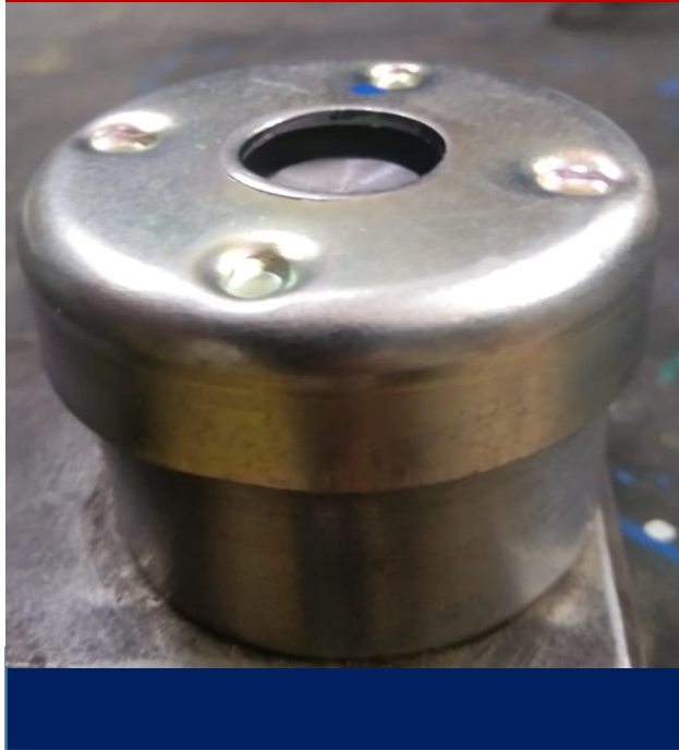
Gauge ID undersize -Gauge wornout
