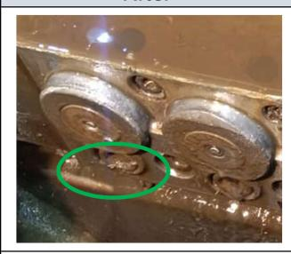
Die locking bolt replaced with new one and tighten.
