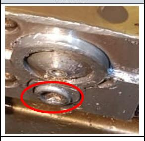
Die locking bolt observed loose in forging 2nd stage
