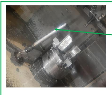
Before: Coolant flow- Pipe Material plastic
