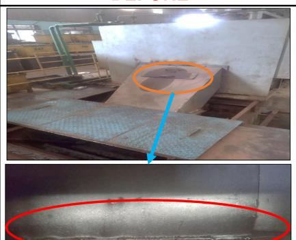
**Remark:** in heat treatment process becouse of this slot all material collected and when model change both material get mixed.
