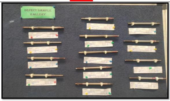
• Earlier No plating peel off defective sample displayed .
