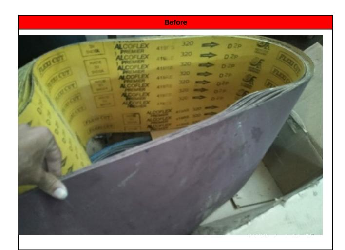
Belt make-Alcoflex Premer (Grit - 320 ) used for deburring
