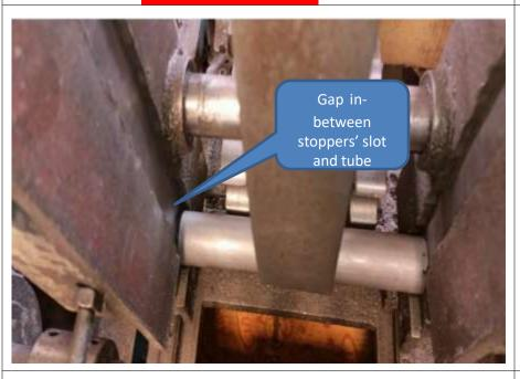
Gap in-between stoppers' slot and tube
