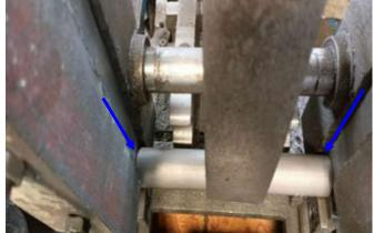
Provide the slot on chamfer machine as a poka yoke, If short length tube insert, It will not clamp and fall down at the below
