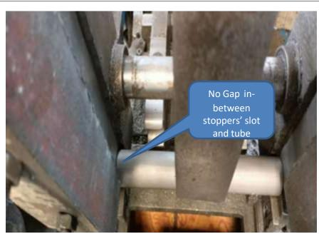
No Gap in-between stoppers' slot and tube
