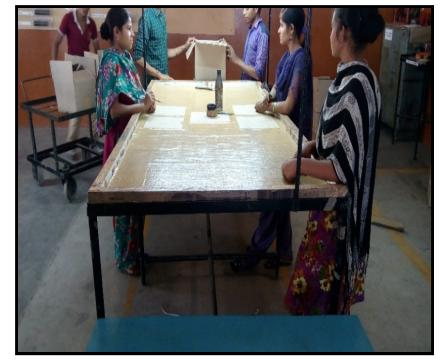
Corrective Action: \*Spring of different model to be start (while model change) only after total completion of previous model till packing. \*Inspector should verify Inspection table duirng model change ie. No where running model spring remain on line and incomplete box to be moved to its appropriate location with identification.
