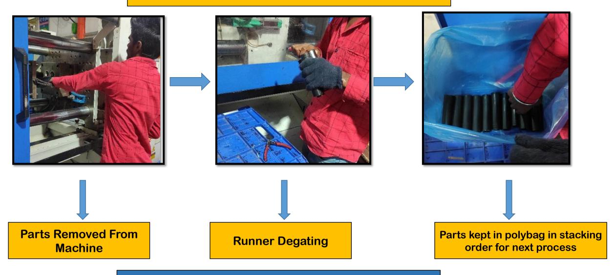
Parts are being placed in polybag in stacking order. No plastic bins are being used for material handling
