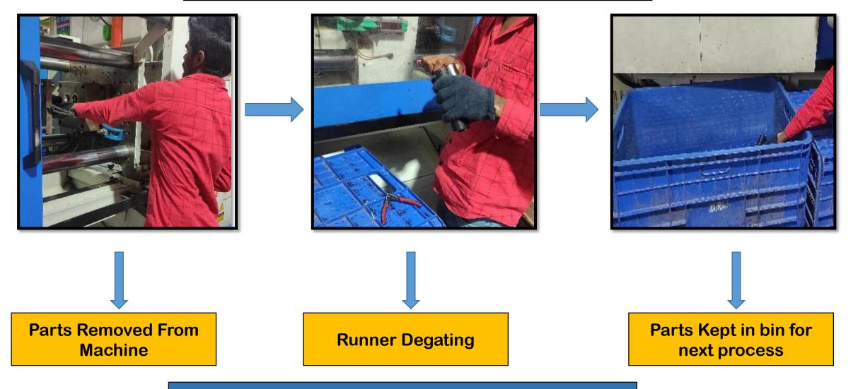
Parts are being placed in bin which are having direct contact resulting in visual defects after handling
