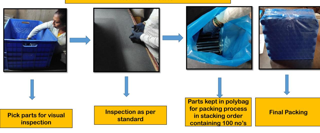
Parts are being placed in polybag in stacking order to avoid any handling defects.
