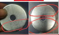
No stamping mark, deep mark OR depth line mark at top surface of Washer K55G.
