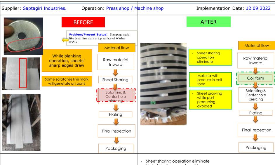
While blanking operation, sheets' sharp edges draw Same scratches line mark will generate on parts
