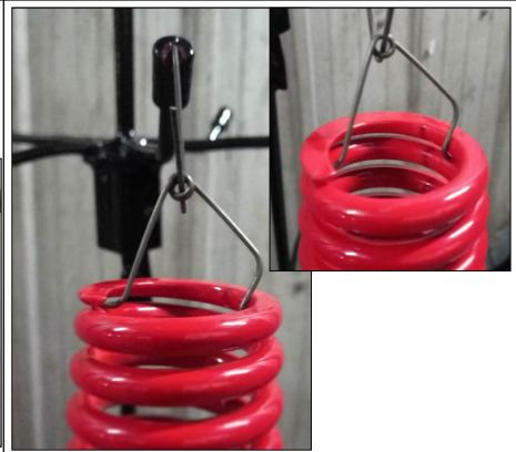
Corrective Action: By hooking with new method hooking hook projection was generated inside face which not get visible after assembly.
