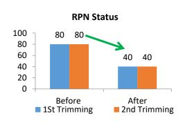
Claw width at 8 places oversize possibility covered in PFMEA at Trimming 1& 2 and adhered(RPN reduced)
