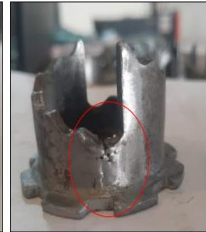
Welding pin hole
