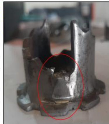
Excess welding ,buffing step
