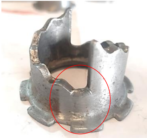
Excess welding ,buffing step
