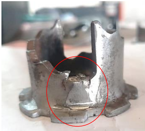
Excess welding ,buffing step
