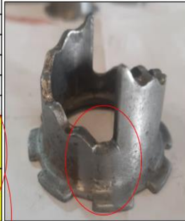
Excess welding ,buffing step
