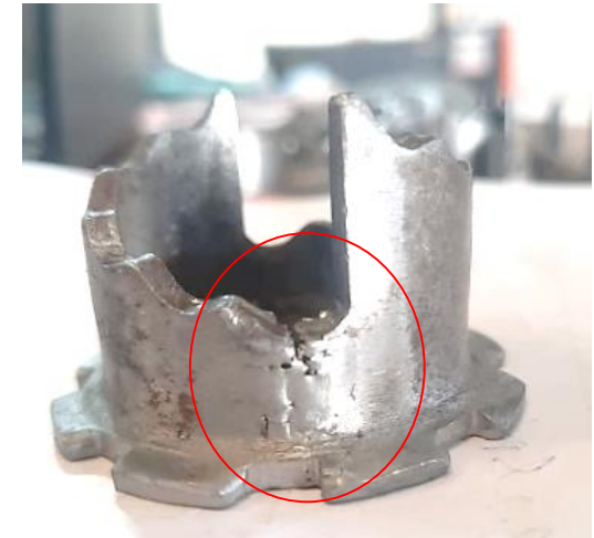
Welding pin hole
