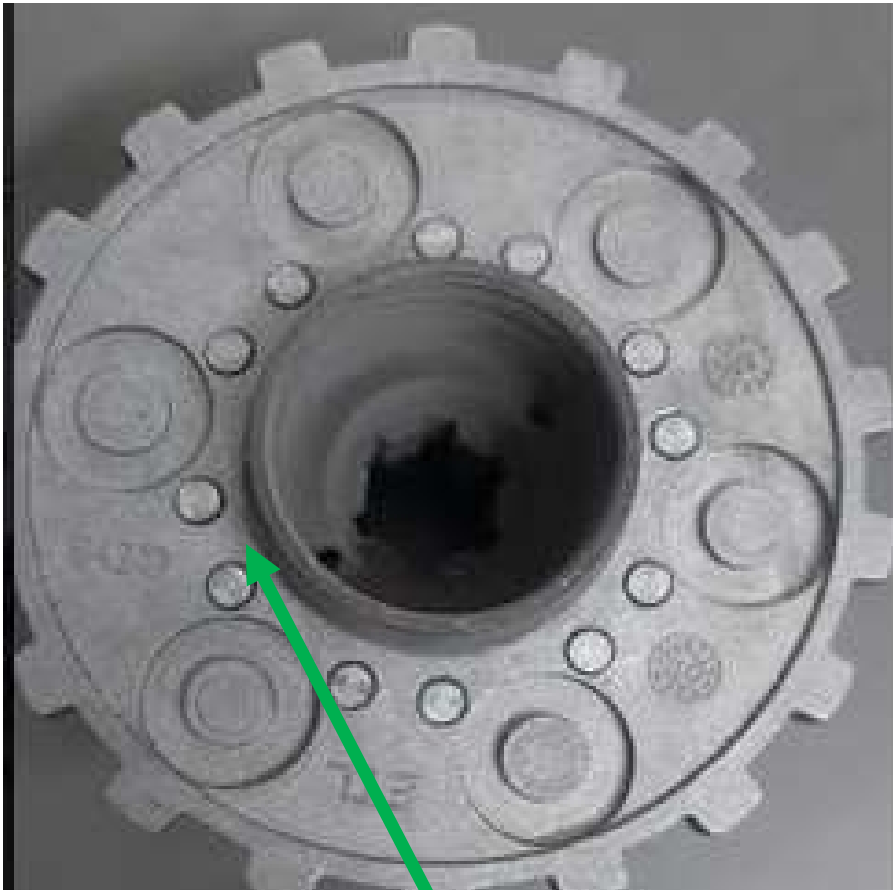
NO CRACK NEAR RIVET
