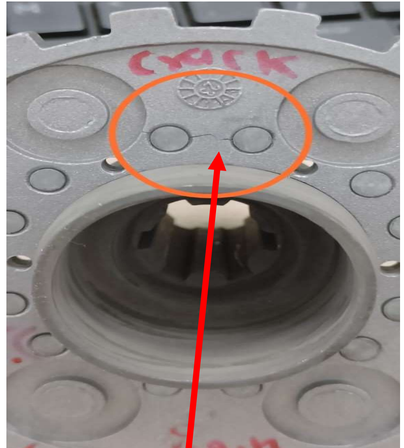
CRACK NEAR RIVET
