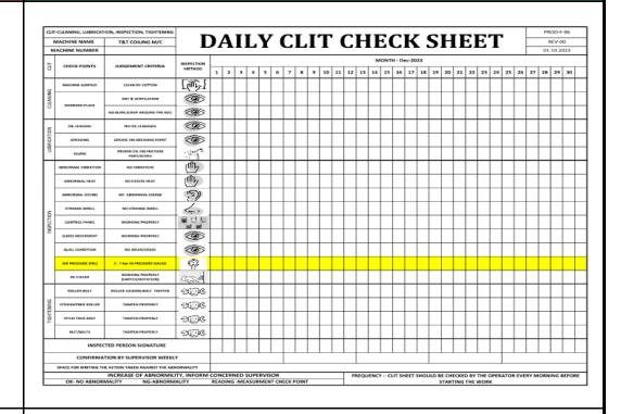
Roller Pressure Check point not Mentioned in check sheet.
