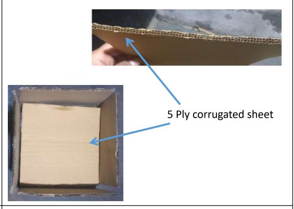
Status: 5 ply extra corrugated sheet provided in box at bottom & top side to avoid Flatness, broken & damage issue in core plate of K70 and as well as in other core plate
