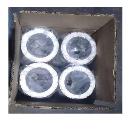
**Status:** 5 ply corrugated box using for core plate packing ,No separator available at bottom & top side ,Change of damage & flatness out issue .
