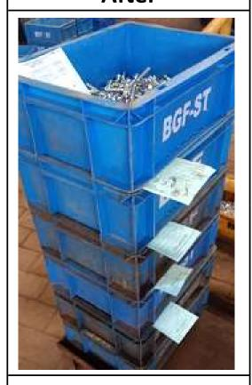
Each material bins identified with identification tag with material number plating stage.
