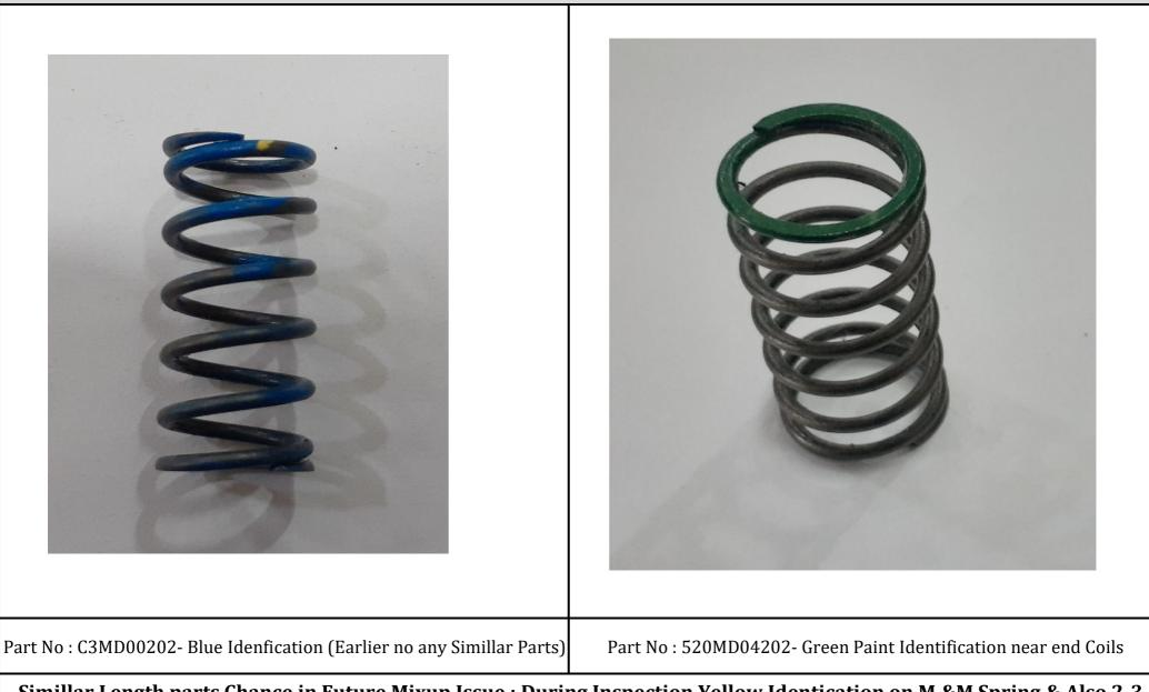
Simillar Length parts Chance in Future Mixup Issue : During Inspection Yellow Identication on M &M Spring & Also 2-3 Days Prodcution gaps to Avoid Inprocess Mixup Issue.
