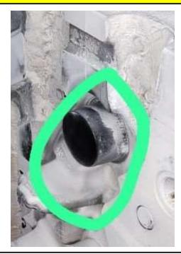
Die Coating Peel of due to touch up time more than 3hrs
