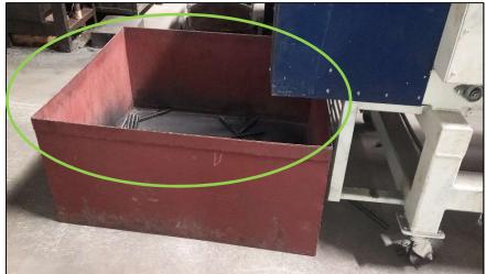
Impact: While line change over when furnace operator goes for material movement another model parts get drop. Small trolley used is not carry enough spring and there arise chance for mix up
