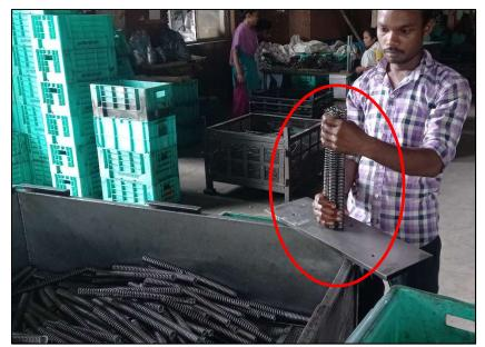
Impact: Free length (mix up) is not checked at final oiling stage
