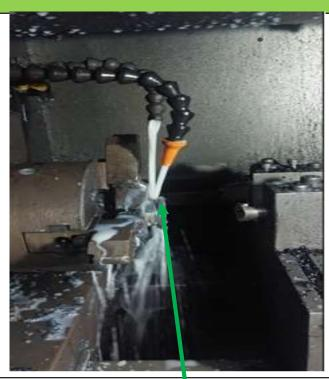
One Coolant Nozzle during machining.
