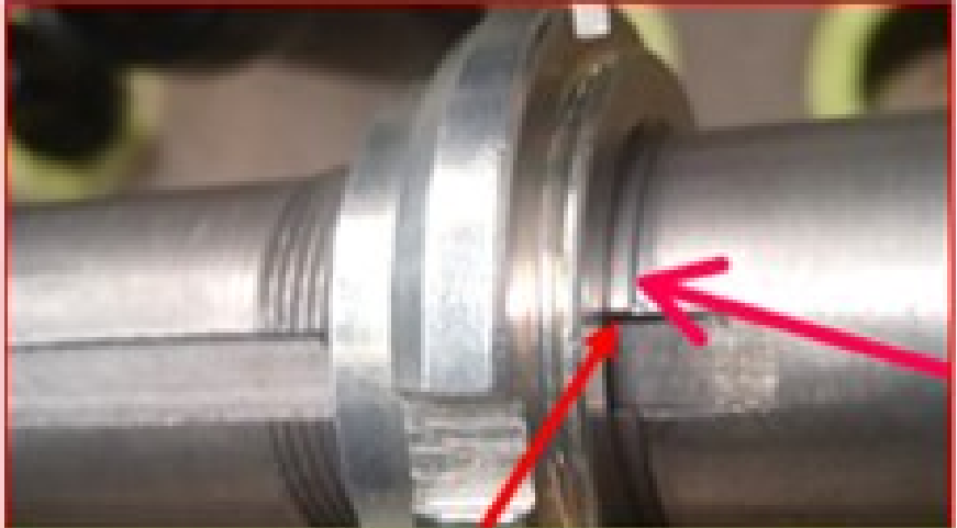
Gap observed after tightening of matting part or Matting part not answering till groove end
