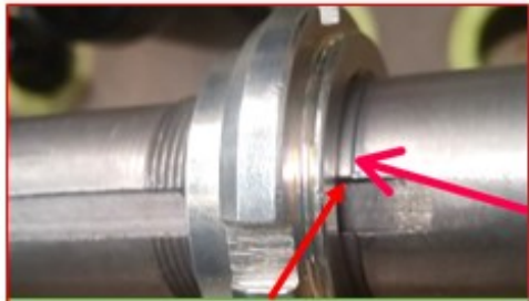
Gap observed after tightening of matting part or Matting part not answering till groove end
