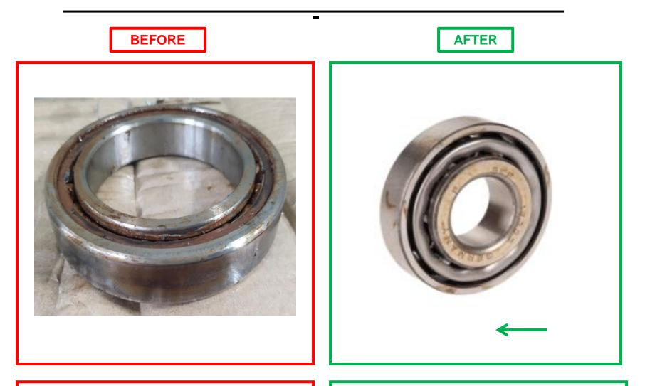
CNC Machine Spindle Bearing Wear out
